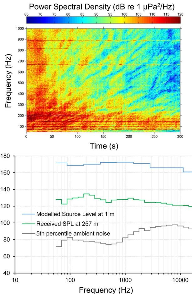
**Fig. 3.** Spectrogram at the closest point of approach for the Awanua in New Zealand (top, distance = 257 m), and its corresponding 1/3-octave spectra along with the estimated source level spectra and 5th percentile ambient noise levels (bottom).
